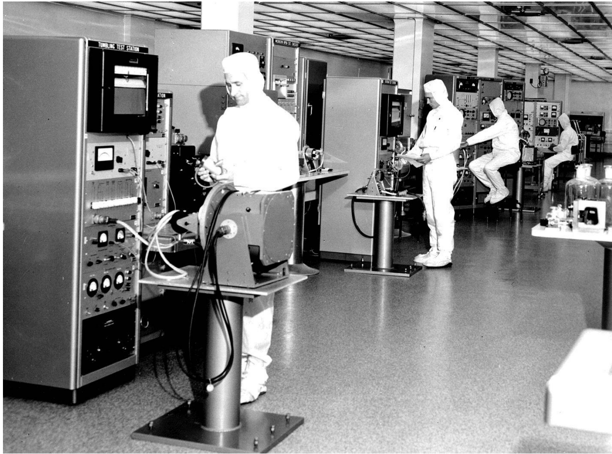
Figure 2. USAF Standard Class IV Clean Room, Downflow. Robins AFB, Georgia. July 1963. (Same design as Figure 1, but air change per hour increased 150 percent.)
