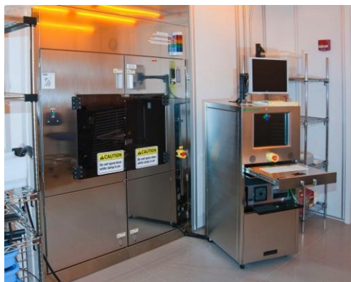
Figure 8—Stepper integration into the wall.
