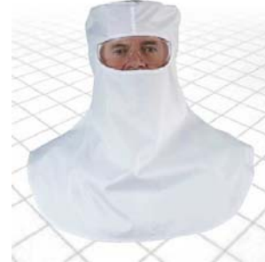
This cleanroom hood uses non-linting, high-density polyester fabric that contains carbon fibers in a grid pattern to control static.
