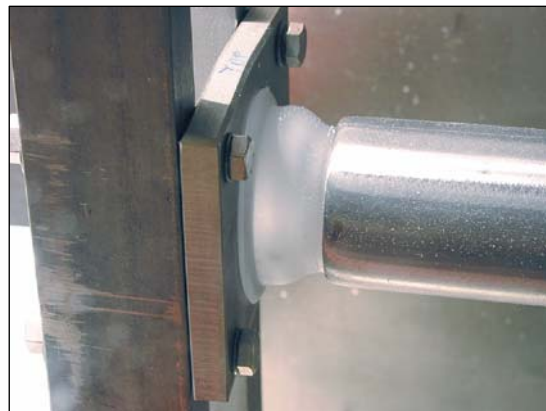
Figure 6. Sabot shown stopped at end of gun barrel. Note that O-rings remain inside barrel to maintain vacuum in the chamber.
