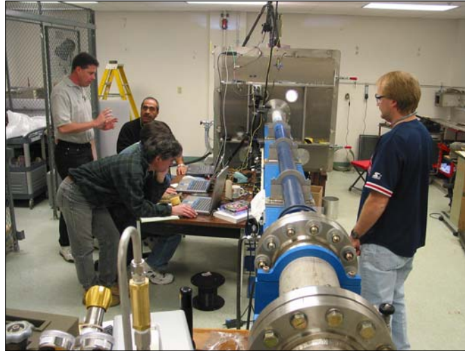
Figure 10. Large vacuum gun with 7.6-cm (3-in.) barrel in GRC Ballistic Impact Lab.
