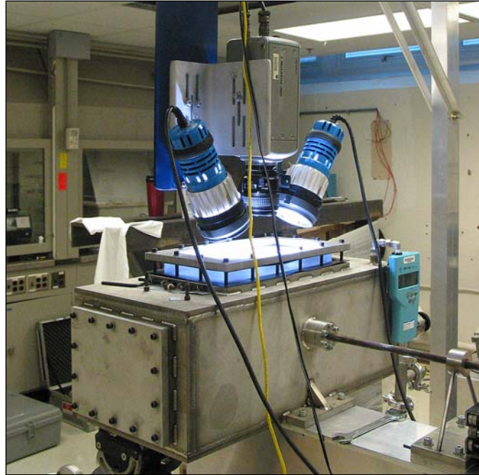
Figure 15. The 0.3175-cm (0.125-in.) vacuum gun with digital camera and lighting system used to shoot 100-450 \mu\text{m} particles at MOR bars.
