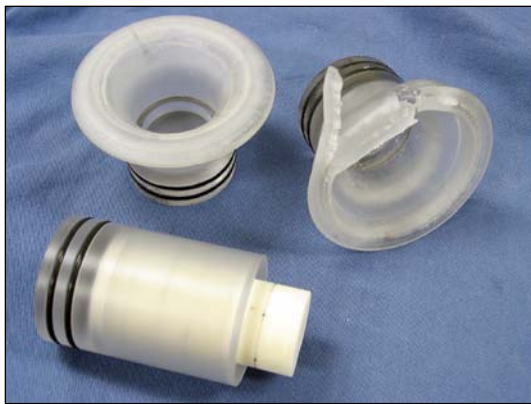
Figure 5. Polycarbonate sabots shown with BX-250 foam projectile in before and after fired condition.
