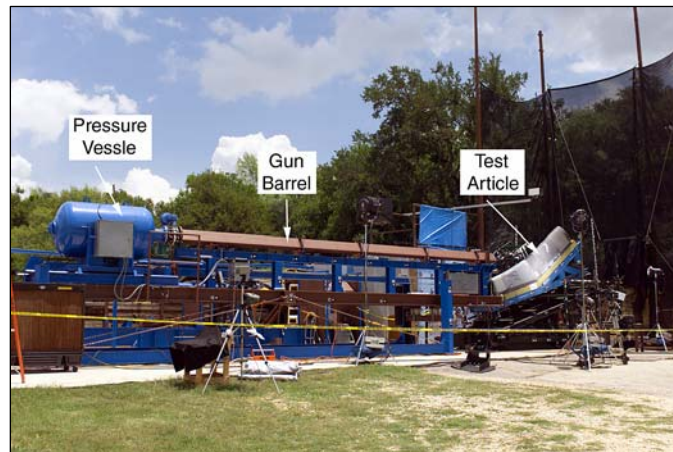
Figure 4. Ballistic test range at Southwest Research Institute shows gas gun and full-scale orbiter leading edge test article.
