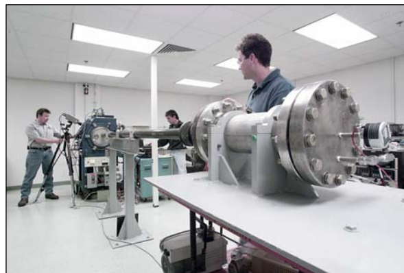
Figure 7. GRC Ballistic Impact Lab small vacuum chamber test setup.
