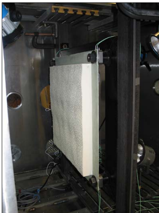
Figure 16. Aluminum test panel with ET TPS foam mounted in large vacuum chamber load frame for 90° impact test.
