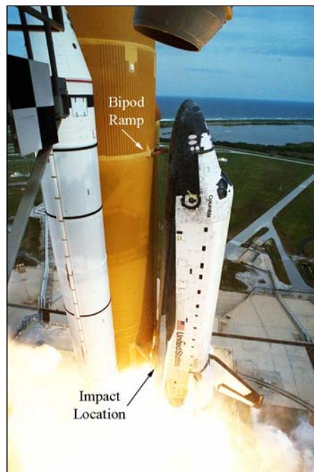
Figure 2. Shuttle Columbia just after liftoff showing the bipod attachment, the bipod ramp, and the location of impact.
