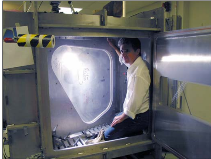
Figure 14. Orbiter window mounted in GRC Ballistic Impact Lab's large vacuum chamber in preparation for test.
